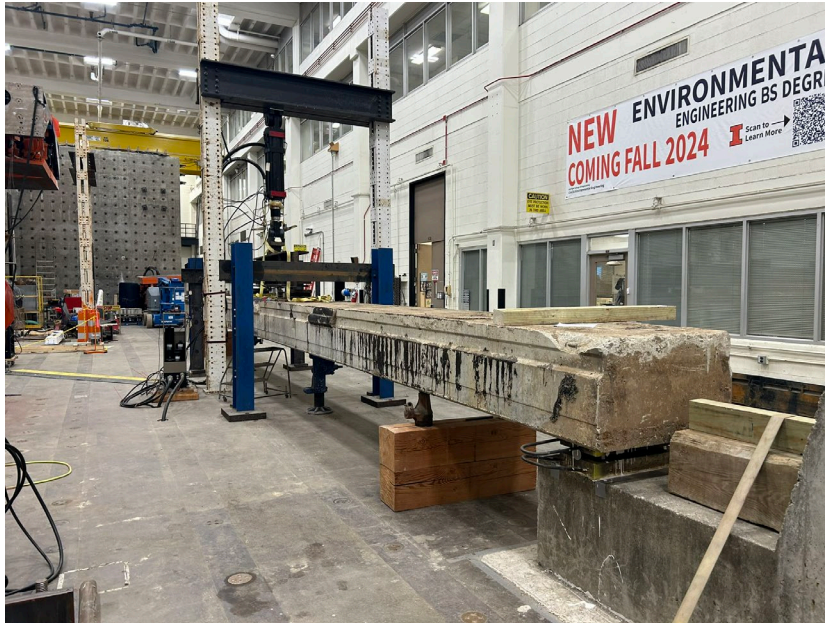
Lab test on a 533mm x914 mm IDOT PPC deck girder beam
