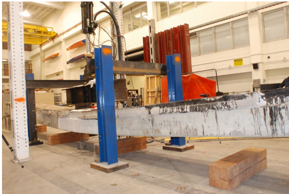
3. Applying load until failure
