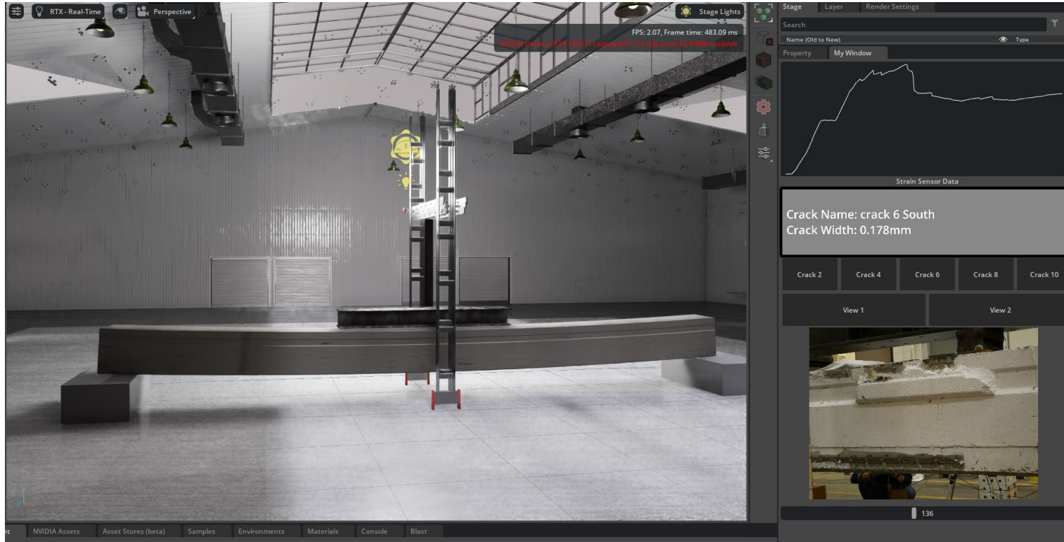
Digital Twin model for Beam testing
